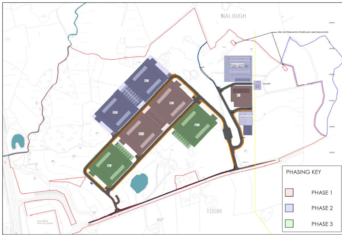
Figure 2.3 Intended Construction Phasing for the proposed Masterplan (ART-ARC-SP-00-DR-A-0003).
