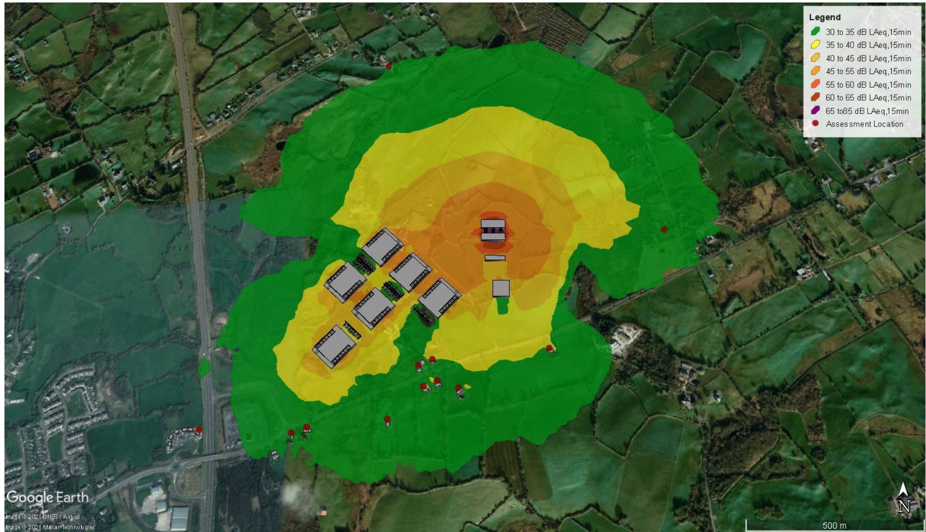
Figure 9.6 Scenario A Proposed Data Storage Facility – Day to Day Noise Contour (Extent of 30dB(A))
